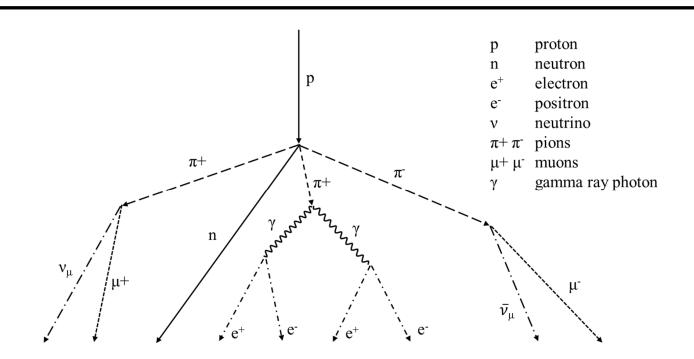
Figure 3: Secondary particles induced by cosmic rays entering the Earth's atmosphere
