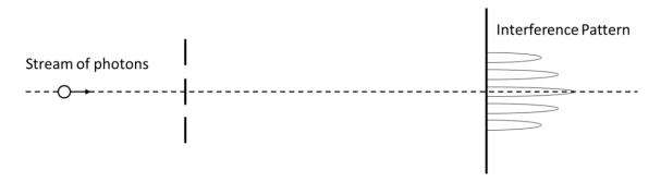
In more recent years this experiment has been performed with single photons (suggesting a particle-like behaviour) and a detector screen. Each photon reaches the screen and the usual interference pattern is gradually built up.
