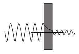
The probability depends on the square of the amplitude. Hence it appears that the electron can 'tunnel out'. This is called quantum tunnelling and has some interesting consequences and possible applications.
