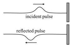
The reflected pulse is said to undergo a phase change of 180° or  $\pi$  radians. The reflected pulse is 180° out of phase with the incident pulse. If these two pulses were to meet they would momentarily cancel as they passed one another.
