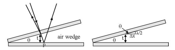
Division of amplitude takes place at the *lower* surface of the top glass slide.
