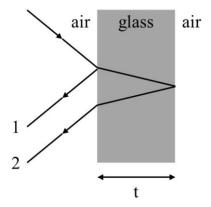
The ray following path 1 reflects off the glass which has a higher refractive index than air. It therefore experiences a  $\pi$  phase change.
