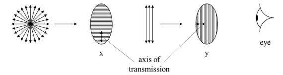
A second polaroid at Y is placed perpendicular to the first one, as shown above. This is called an **analyser**. The analyser absorbs the remaining vibrations because its axis of transmission is at right angles to the polariser at X and no light is seen by the eye. The light between X and Y is called **linearly** or **plane polarisation**.
