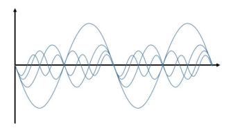
When all these terms are superimposed (added together) the graph below is obtained. Notice that this is tending to the saw tooth waveform. If more terms are included it will have a better saw tooth form.
