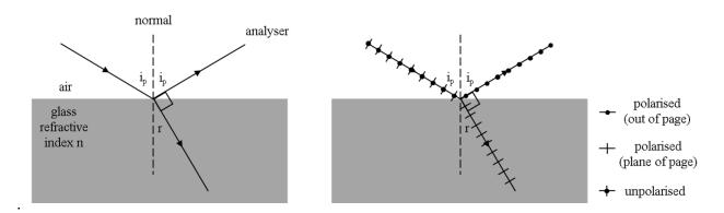
Consider a beam of unpolarised light incident on a sheet of smooth glass. This beam is partially reflected and partially refracted. The angle of incidence is varied and the reflected ray viewed through an analyser, as shown above. It is observed that at a certain angle of incidence ip the reflected ray is plane polarised. No light emerges from the analyser at this angle.
