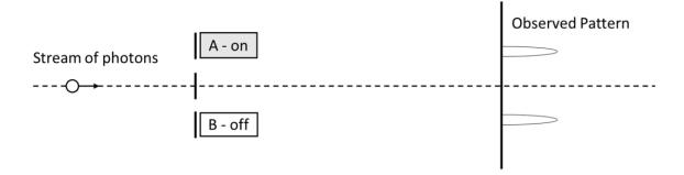
We lose the interference effect and simply obtain a pattern for particles passing through two slits. We would get the same pattern if we switched on detector B instead of detector A or if we switched on both detectors.
