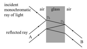
Notice that an **extended** source can be used. The amplitude of the beam is divided by reflection and transmission at D1, and again by reflection and transmission at D2 at the back of the glass sheet.
