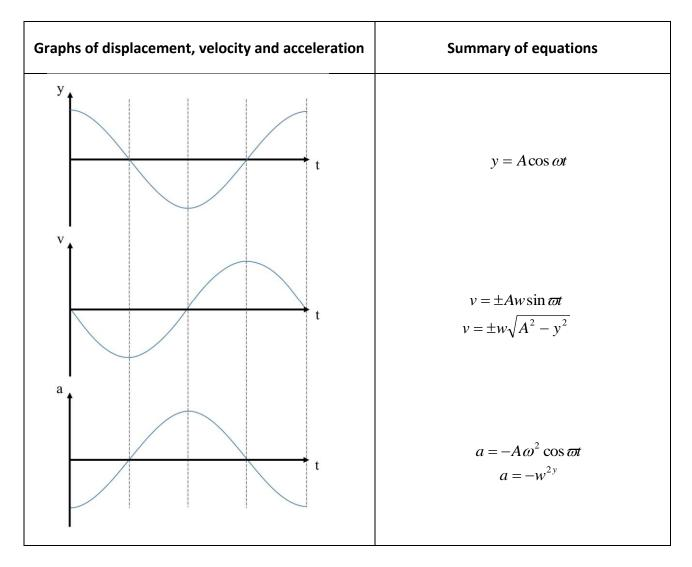
Note that this form, acceleration = -  $\omega^2$  y, is consistent with our definition of SHM,  $\omega^2$  is a positive constant. This implies that the sine and cosine equations must be solutions of the motion.
