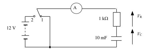
The switch is in position 1 and the capacitor is uncharged. The switch is now moved to position 2 and the capacitor charges. The graphs show how  $V_{\rm C}$ , the p.d. across the capacitor, and  $V_{\rm R}$ , the p.d. across the resistor, vary with time.
