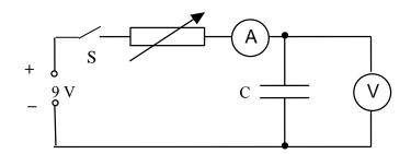
Switch S is now closed. By carefully adjusting the variable resistor R a constant charging current of 1.0 mA is maintained.
