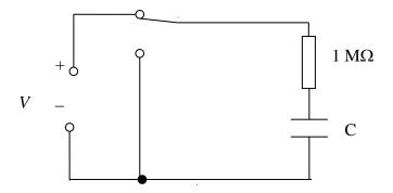
C is either a single capacitor or two capacitors in series. The table shows the resistance of R, the capacitor arrangement used and the value of the time constant.
