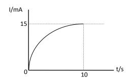
A milliammeter is used to monitor the current in the circuit. The switch is now closed. The graph shows the variation of current with time.
