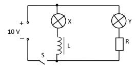
The supply has negligible internal resistance. The rating of each lamp is 6.0 V, 3.0 W.
