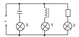
The a.c. supply is of constant amplitude but variable frequency. The frequency of the supply is varied from a very low frequency to a very high frequency.
