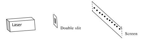
Calculate the separation of the bright fringes on a screen placed 0.92 m beyond the double slit.
