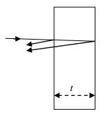
The two reflected rays can interfere constructively or destructively.
