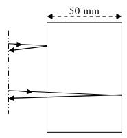
The perspex block has a refractive index of 1.47 and a thickness of 50 mm.
