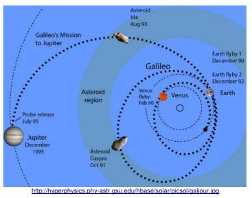
This was done by flying the probe past Venus and using the **planet's gravitational field** to *sling shot* it with increased speed. The process was then repeated using the Earth's gravitational field (twice) before the probe had enough speed to reach Jupiter.
