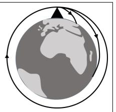
This would then be a satellite. The object remains in orbit because <u>it is being pulled</u> to the Earth by gravity, NOT because it has *escaped gravity*.
