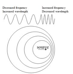
Similarly **fewer sound waves** are received per second when the source of sound waves is **moving away** from the observer and so the frequency heard by the observer is **decreased**.
