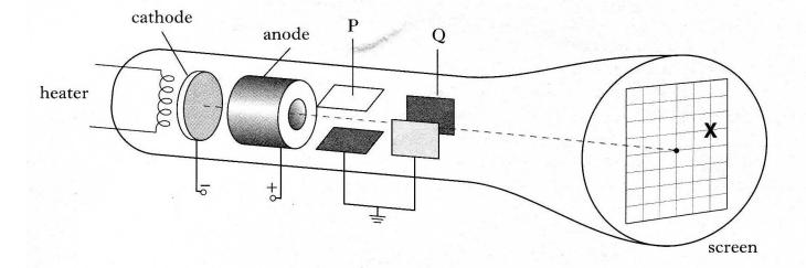
The diagram below shows a cathode ray tube used in an oscilloscope.
