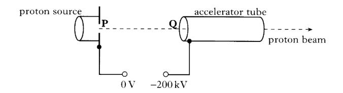
Protons released from the proton source start from rest at  $\mathbf{P}$ . A potential difference of 200 kV is maintained between  $\mathbf{P}$  and  $\mathbf{Q}$ .
