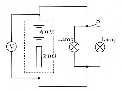
Describe and explain what happens to the reading on the voltmeter when switch S is closed.
