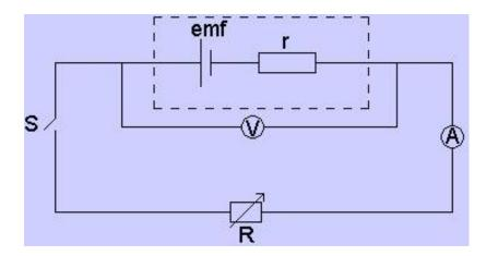
In the circuit above, the switch is closed for a short time. The readings are then recorded from the **ammeter** and the **voltmeter** and shown **in the table below**.
