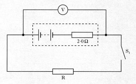
The internal resistance of the battery is  $2 \cdot 0 \Omega$ .
