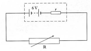
The graph below shows how the "lost volts" of this battery changes as the resistance of R increases.
