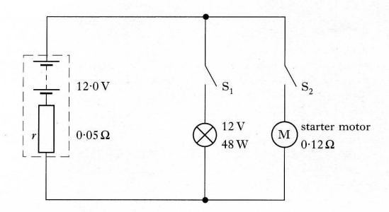
The battery has an e.m.f. of  $12.0 \,\mathrm{V}$  and an internal resistance r of  $0.05 \,\Omega$ . The battery is connected across a  $12 \,\mathrm{V}$ ,  $48 \,\mathrm{W}$  headlamp and a starter motor of resistance  $0.12 \,\Omega$  as shown.
