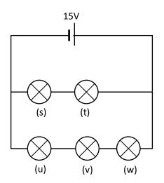
2. In the following circuits the bulbs are identical. Calculate the current through each lettered bulb.
