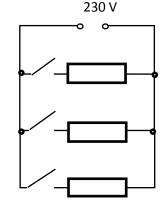
6. The headlamps and side lights in a car are connected in parallel. The diagram below shows how they are connected. The side lights  $(L_1 \& L_2)$  may be switched on by themselves using switch S<sub>1</sub>. The headlights  $(H_1 \& H_2)$  are switched on by switch S<sub>2</sub> and only come on if the sidelights are already on.
