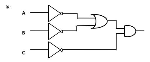
5. Each of the following combinations of logic gates involve linked inputs, that is two inputs being fed into different gates. For each combination complete a truth table of the form:
