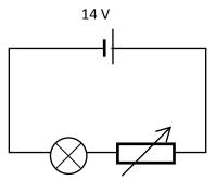
The variable resistor is adjusted until the bulb is shining brightly. The voltage across the bulb is 13.8 V and the current through the variable resistor at this setting is 1.7 A.
