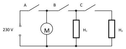
The motor draws a current of 3 A from the mains and the heating elements draw a current of 2 A each from the mains.
