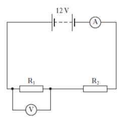
The reading on the ammeter is  $3.0\,\mathrm{A}$ . The reading on the voltmeter is  $4.0\,\mathrm{V}$ . Which row in the table shows the current in resistor  $R_2$  and the voltage across resistor  $R_2$ ?
