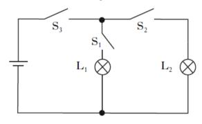
Which switch or switches must be closed to light lamp  $L_1$  only?
