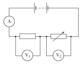
If the resistance of the variable is increased, what happens to the readings on the three meters?
