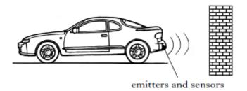
Ultrasonic pulses, which travel at  $340 \text{ms}^{-1}$ , are emitted from the rear of the car. Objects behind the car reflect the pulses, which are detected by sensors. The time between pulses being emitted and detected is  $2 \times 10^{-3}$ s. Calculate the distance between the object and the rear of the car.
