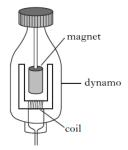
When the magnet spins, a voltage is induced in the coil.
