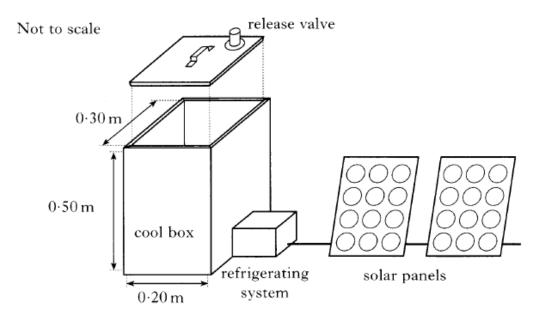
The lid is placed on a cool box with the release valve closed. An airtight seal is formed. When the lid is closed the air inside the cool box is at a temperature of  $33^{\circ}$ C and a pressure of  $1.01 \times 10^{5}$ Pa.
