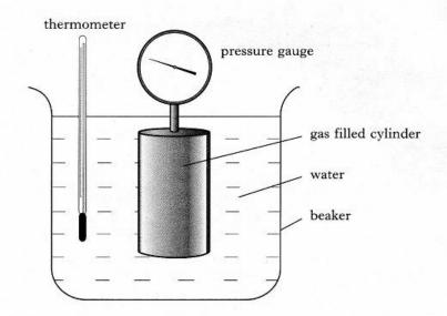
The cylinder is fully immersed in a beaker of water and the water is slowly heated. You may assume that the volume of the cylinder does not change as the temperature of the water changes.
